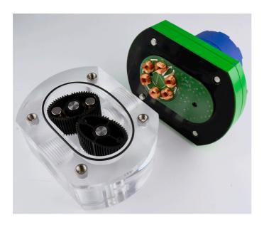
Energy-independent flow measurement system with remote read-out © Fraunhofer IIS/Heiko Wörrlein | Picture in color and print quality: www.iis.fraunhofer.de/pr.
